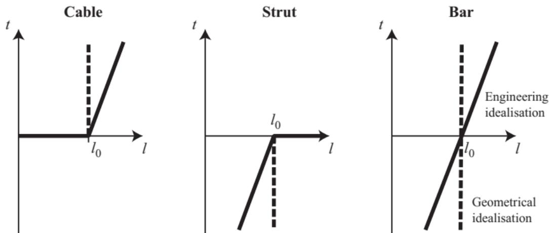
In a purely geometric construction, the members are infinitely stiff. An engineer might assume that the members have some stiffness  $k$ , and:
