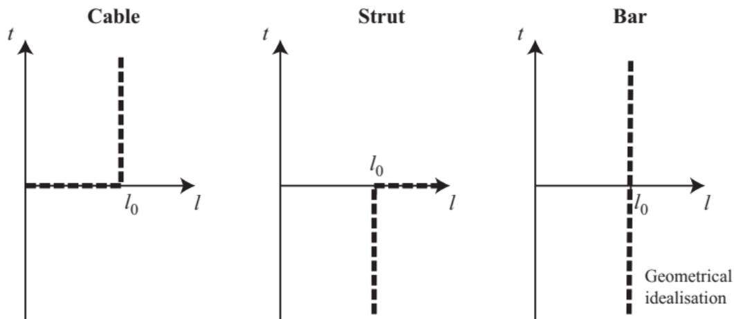
In a purely geometric construction, the members are infinitely stiff.
